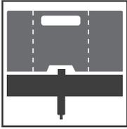
Insert the Tannus Tubeless Fusion inside the tire and make sure it is properly aligned throughout the full length of the tire.
