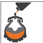
Deflate the tire and add the sealant through the valve stem into the tire. *(Please use Tannus sealant or similar sealant to avoid sealants that have solvents).*
