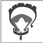
Push both sides of the Tannus Tubeless insert into the rim before mounting the second tire bead.
