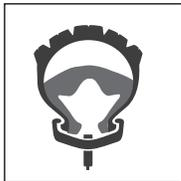
Mount the second bead on the rim. Make sure that the first bead is pushed into the center channel of the rim to make the installation easier.
